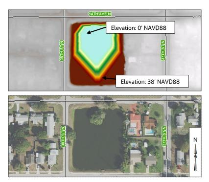
Figure 4-6. DEM Error with Artificially Low Elevations within a Pond, Excessive Elevation Difference
